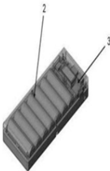
Fig.2: Inner view of solar cum electric power bank
